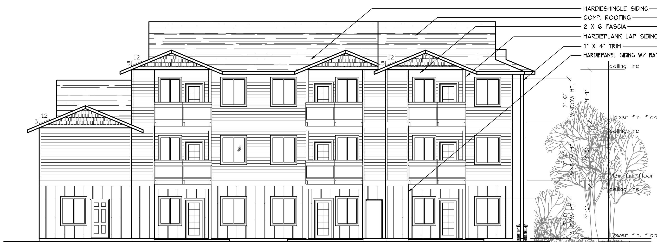
SOUTH ELEVATION (TYPE C UNITS) SCALE: 1/8" = 1'-0" BLD. 2
