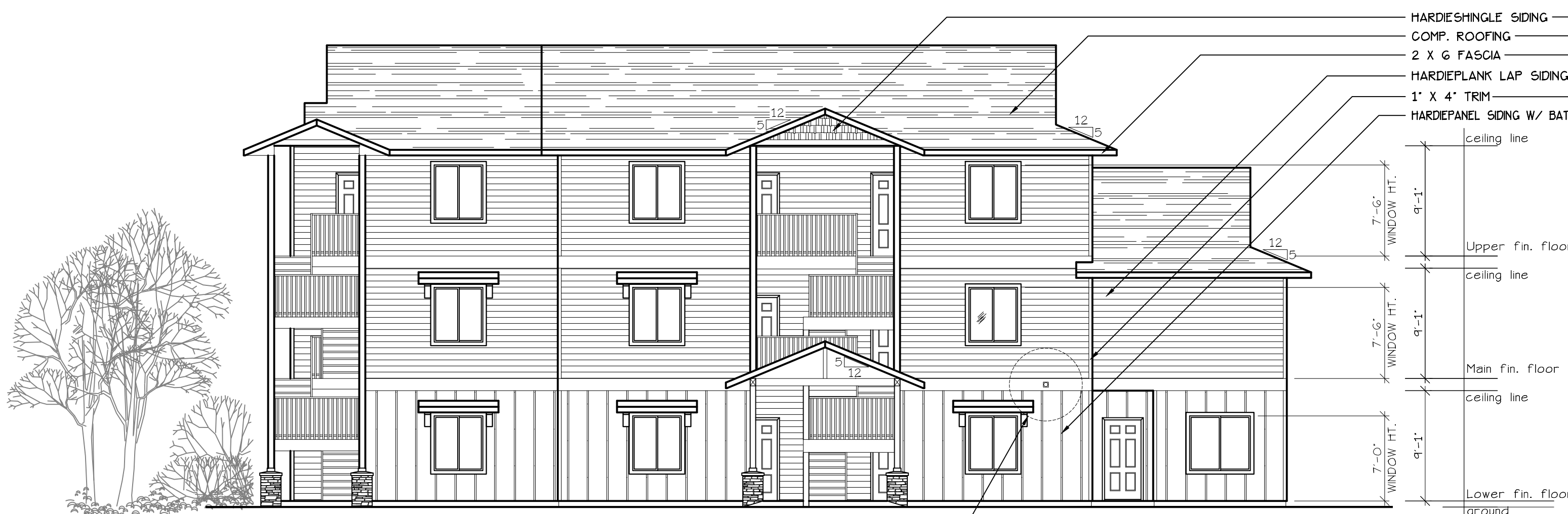
NORTH ELEVATION (TYPE C UNITS) SCALE: 1/8" = 1'-0" BLD. 2
