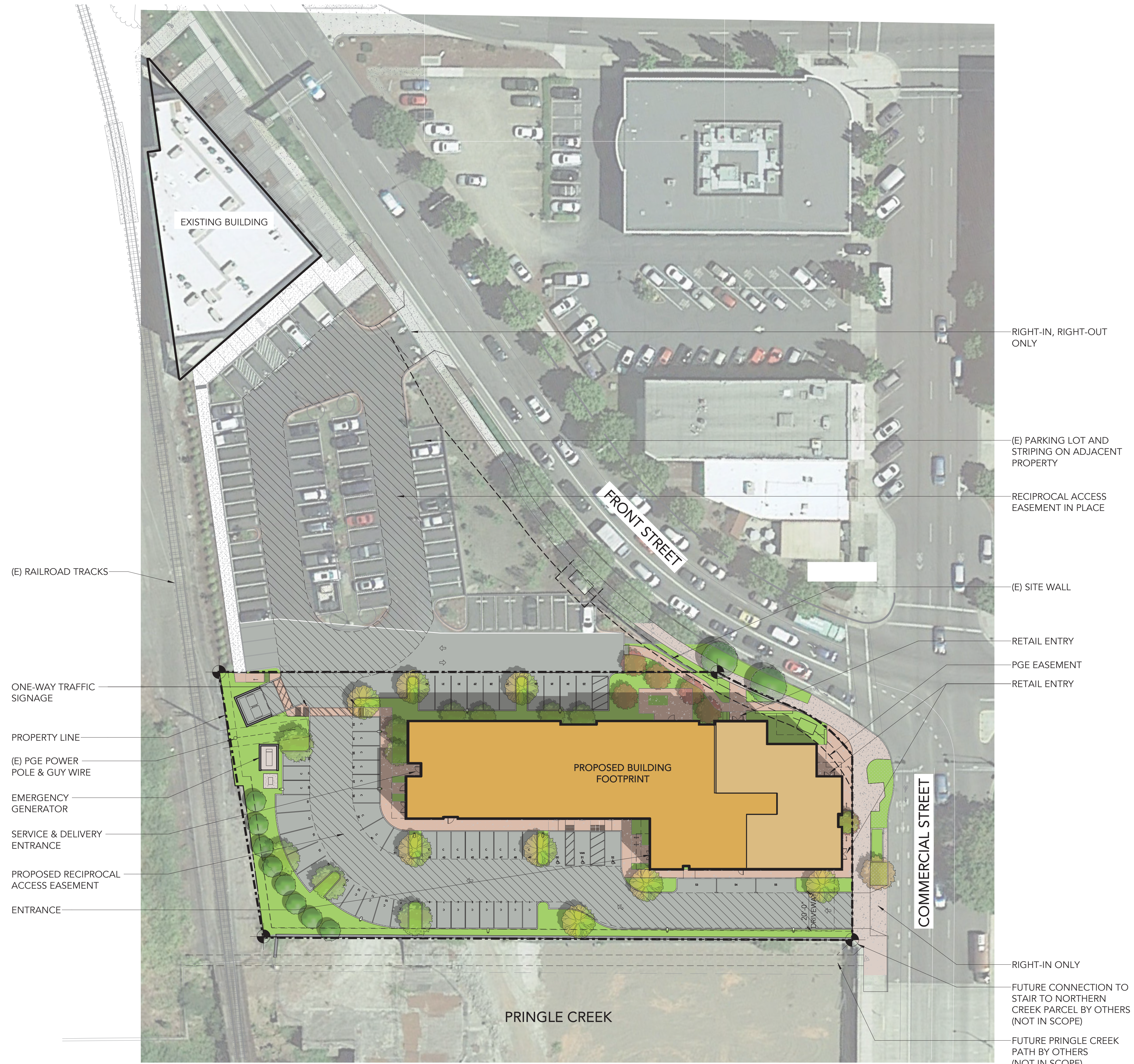
OVERALL SITE PLAN SCALE: 1" = 30'-0"
