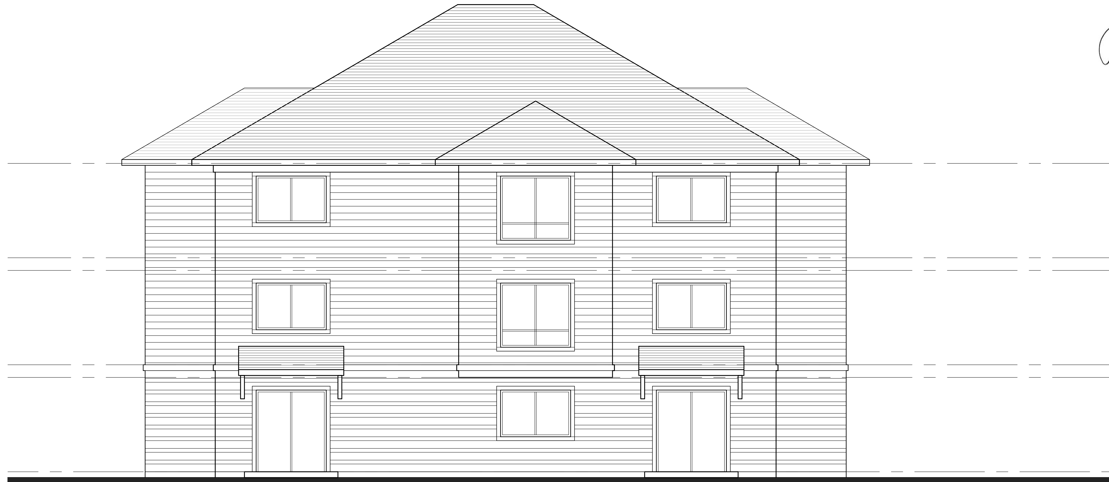
2 STREET ELEVATION - 12 PLEX 1/4" = 1'-0" SEE TYPICAL NOTES 1/A200
