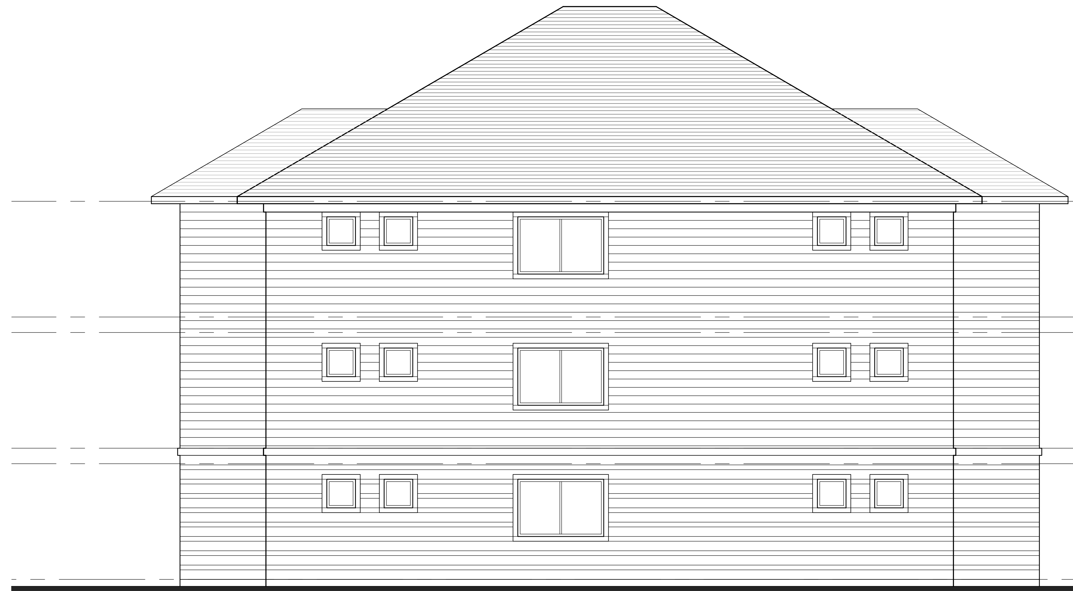
2 SIDE ELEVATION - 12 PLEX 1/4" = 1'-0" SEE TYPICAL NOTES 1/A203
