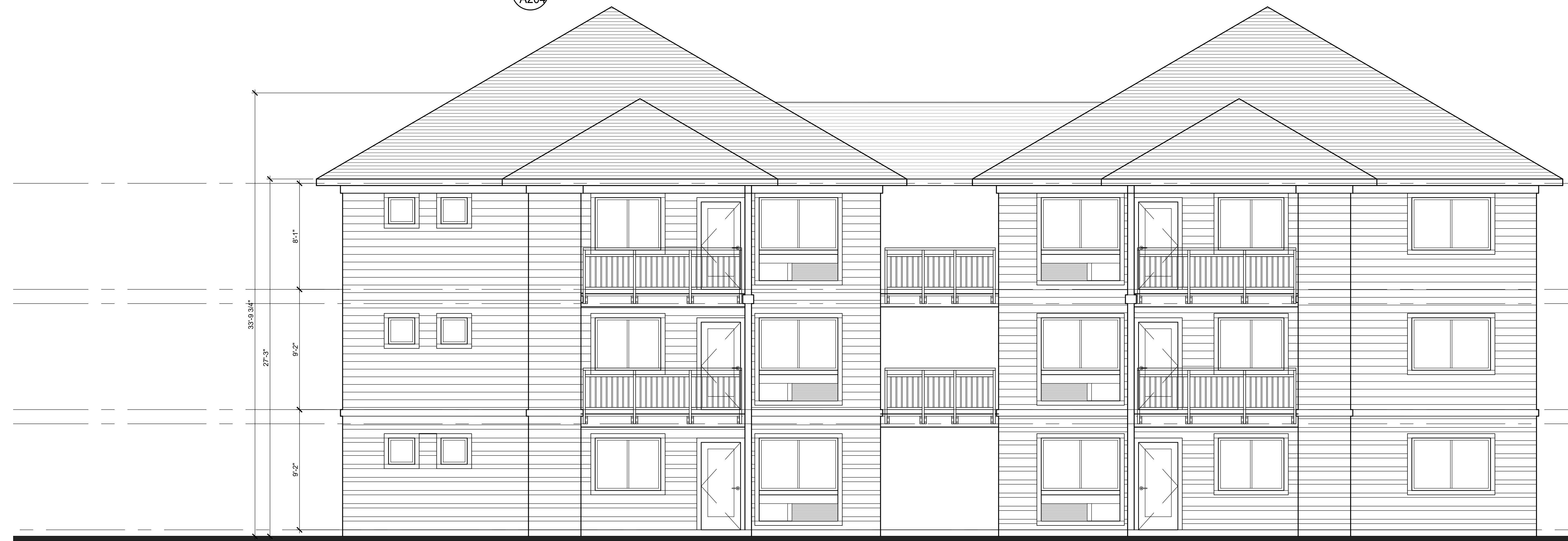
1 BACK ELEVATION - 12 PLEX 1/4" = 1'-0" SEE TYPICAL NOTES 1/A203
