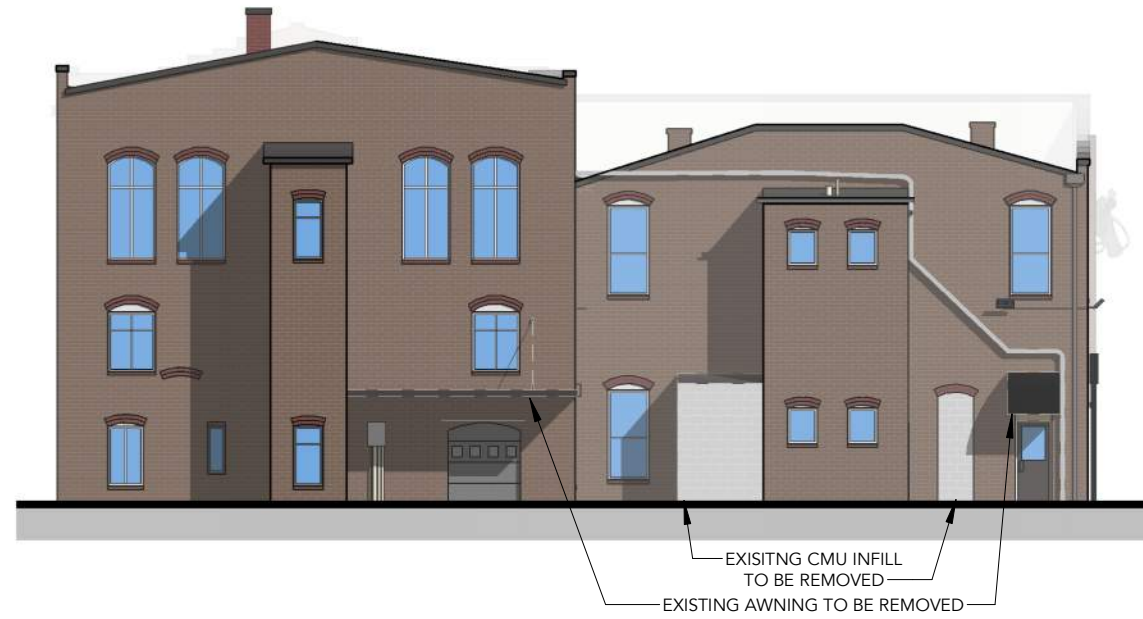
NORTH ELEVATION - EXISTING
