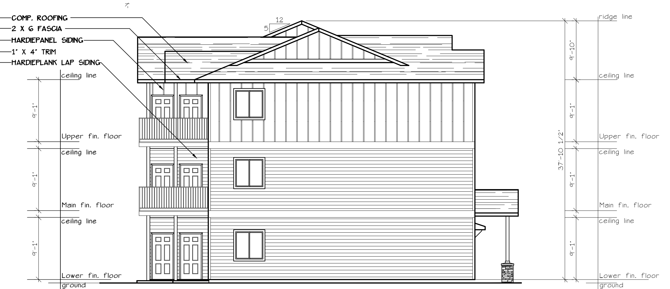
SOUTH ELEVATION (TYPE D UNITS) SCALE: 1/8" = 1'-0" (BLD. 1.4.16.17.18.+35)
