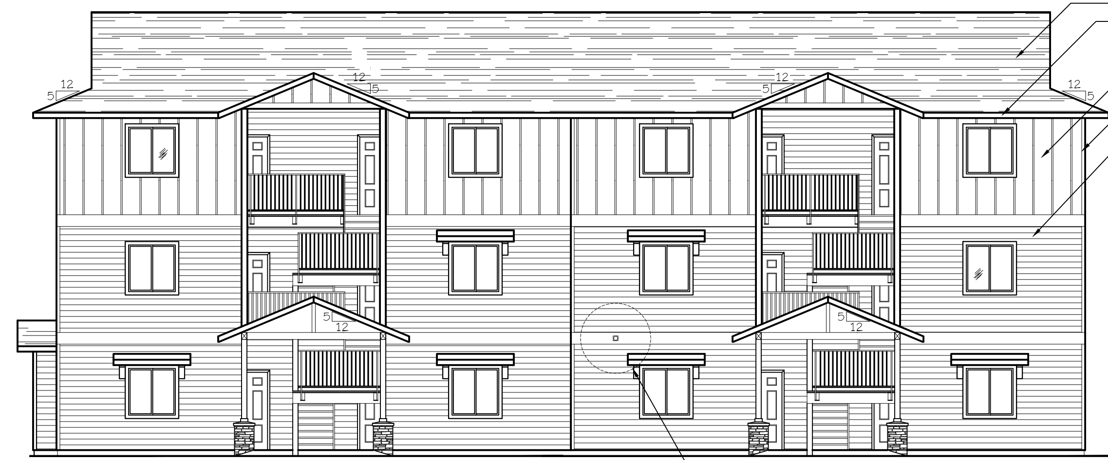
EAST ELEVATION (TYPE E UNITS) SCALE: 1/8" = 1'-0" BLD. 27
