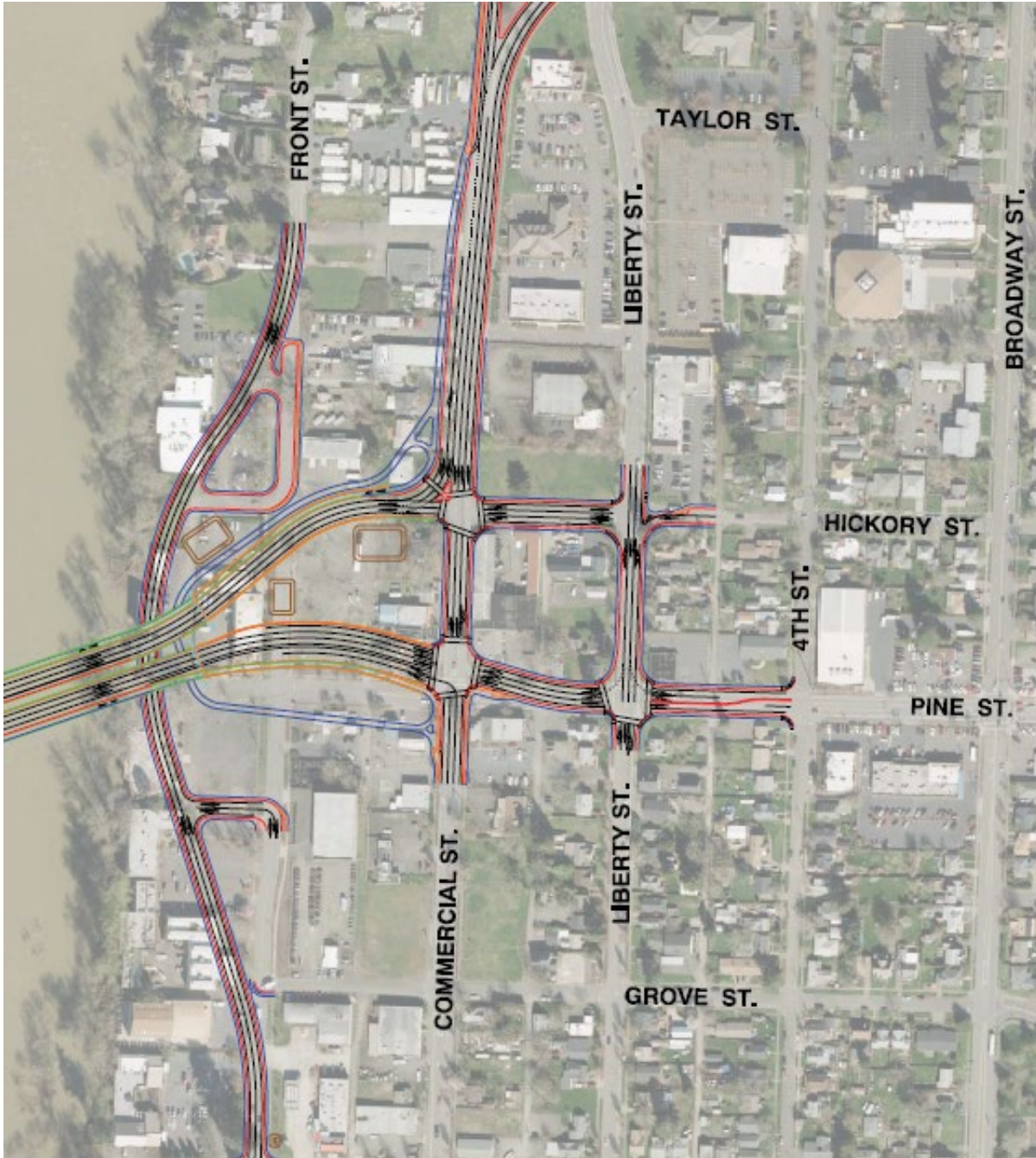
Figure 12: Preferred Alternative – Eastside Bridgehead and Distribution Network (Multi-Use Path Shown in Blue Outline)
