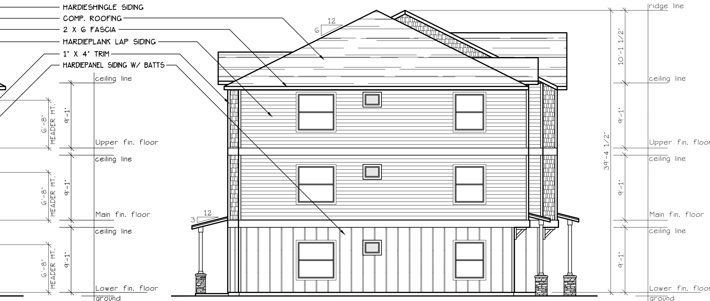
SOUTHEAST ELEVATION (TYPE A UNITS) SCALE: 1/8" = 1'-0" BLD. 1+2
