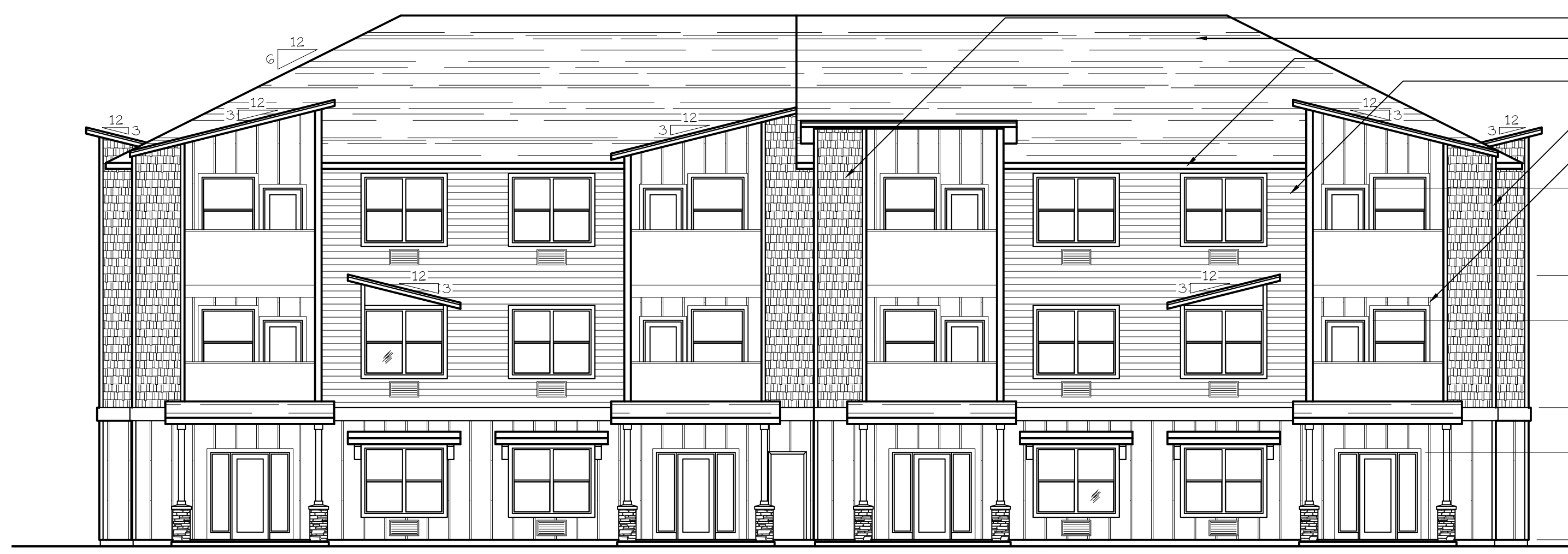
REAR ELEVATION (TYPE B UNITS) SCALE: 1/8" = 1'-0" BLD. 3,4,8,9,11-17
