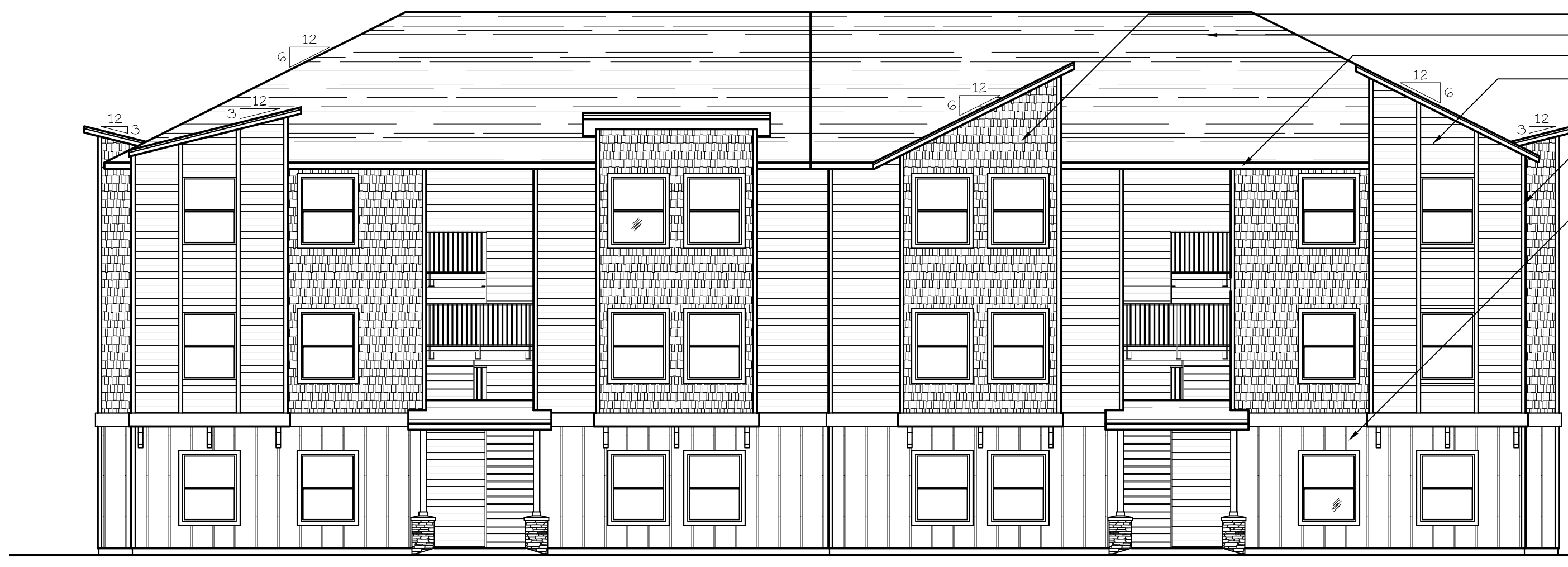
WEST ELEVATION (TYPE B UNITS) SCALE: 1/8" = 1'-0" BLD. 19+23
