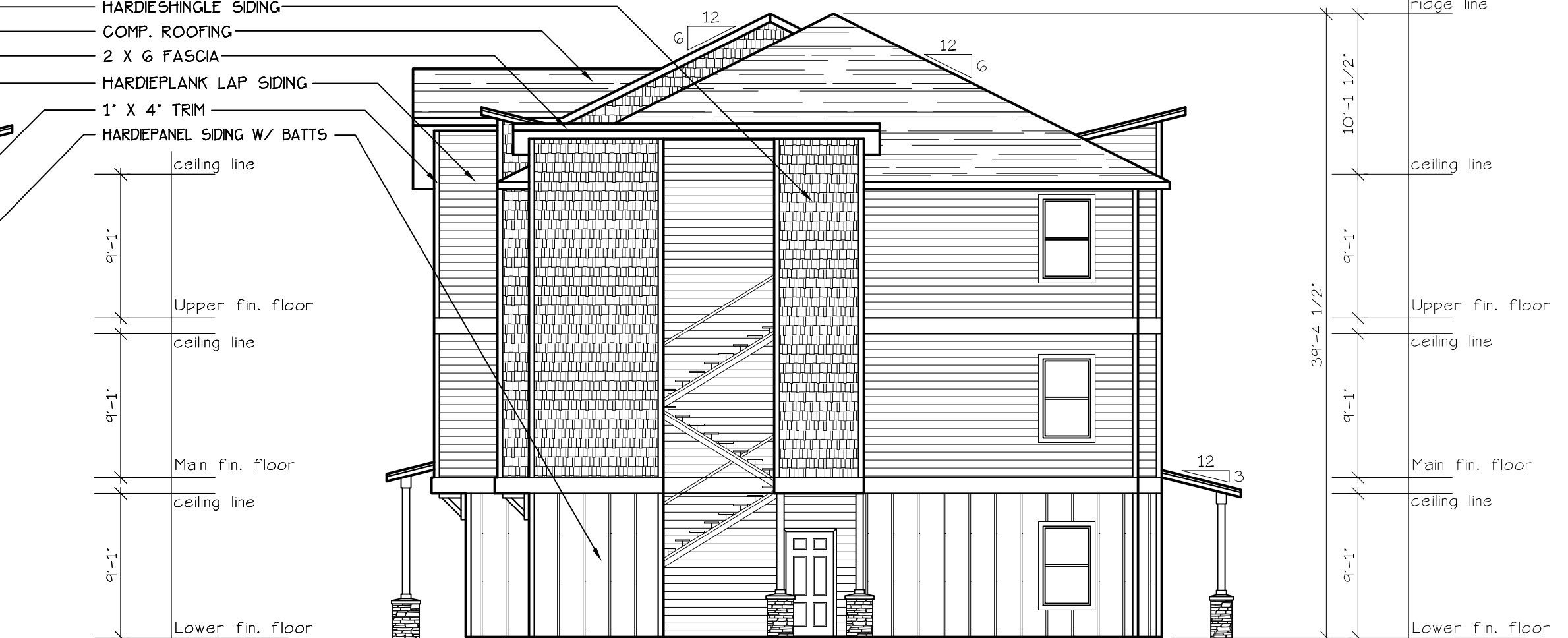
NORTHWEST ELEVATION (TYPE A UNITS) SCALE: 1/8" = 1'-0" BLD. 1+2
