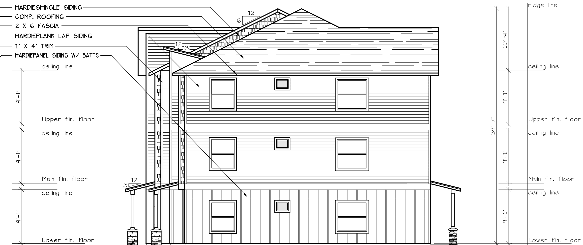
EAST ELEVATION (TYPE C UNITS) SCALE: 1/8" = 1'-0" BLD. 2
