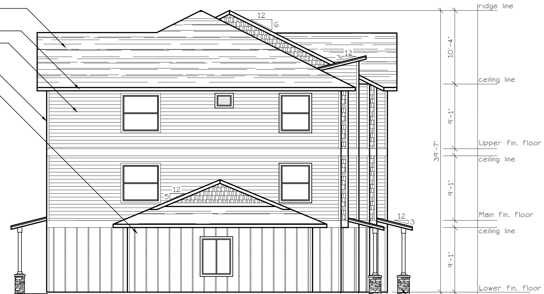
WEST ELEVATION (TYPE C UNITS) SCALE: 1/8" = 1'-0" BLD. 1
