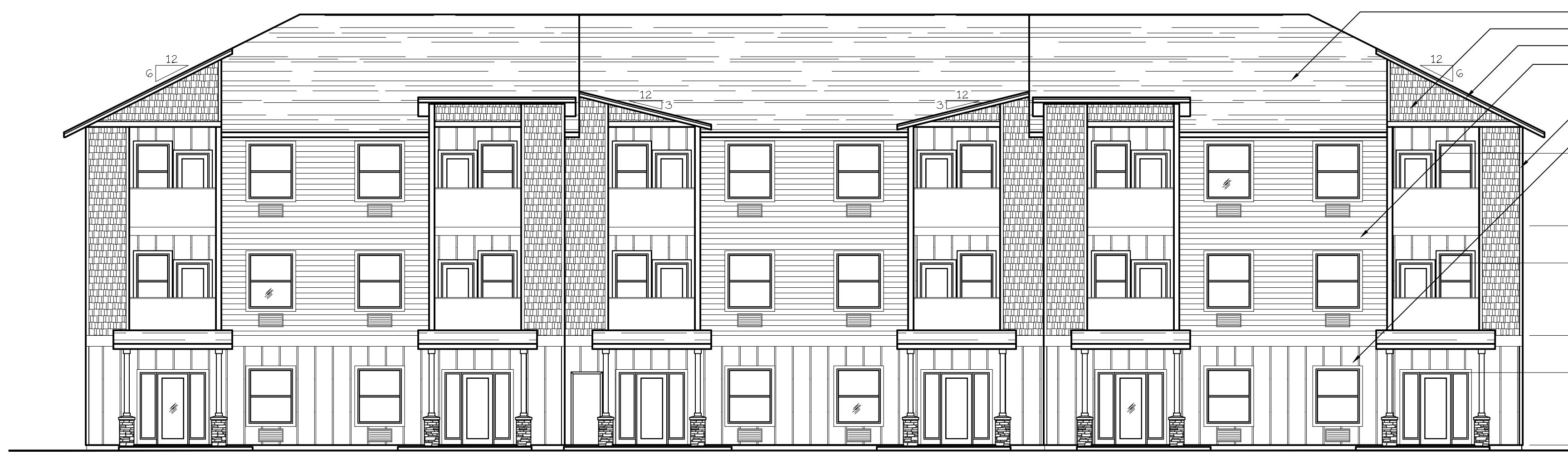
NORTH ELEVATION (TYPE C UNITS) SCALE: 1/8" = 1'-0" BLD. 2
