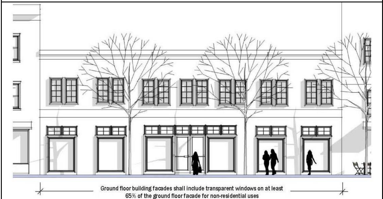
FIGURE 534-4 GROUND FLOOR WINDOWS
