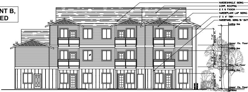
SOUTH ELEVATION (TYPE C UNITS) SCALE: 1/8" = 1'-0" BLD. 2
