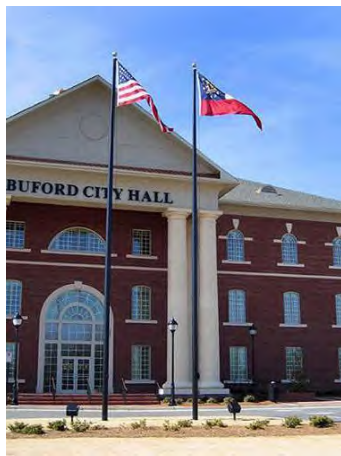
FLAG POLE Cast Aluminum Pole Product: Concord American 'Contnetal ESR-40' Color: Powdercoated Black Height: 40'
