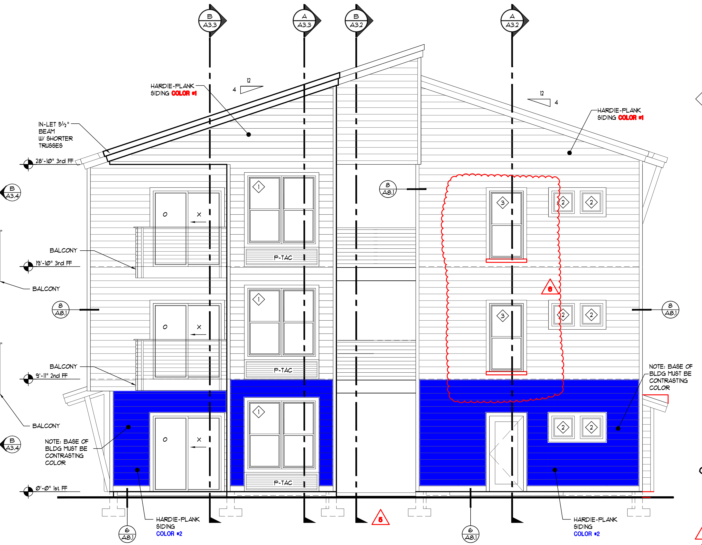
SOUTH-BUILDING "A" EAST ELEVATION SCALE: 1/4" = 1'-0"
