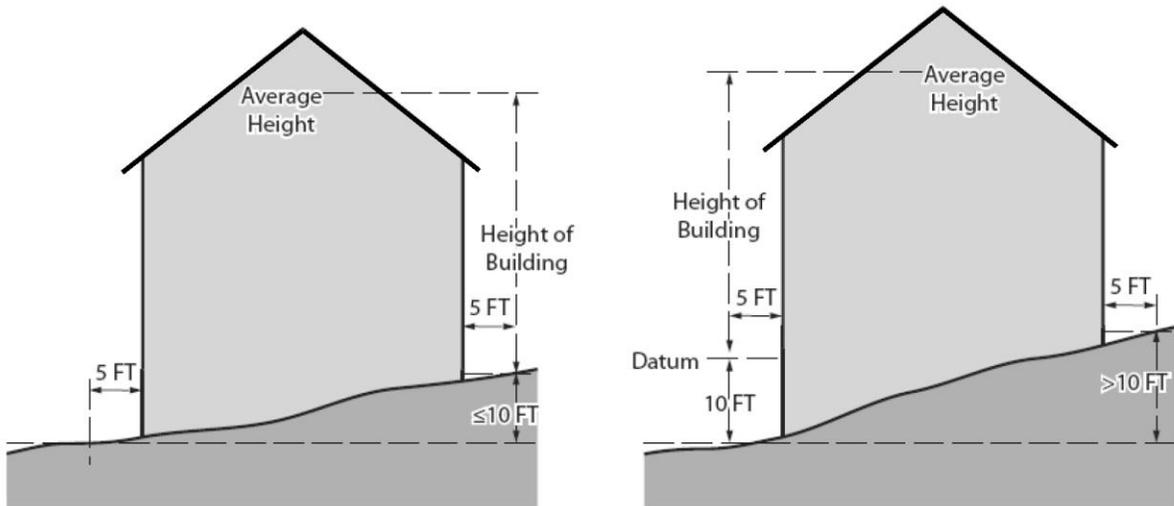
FIGURE 112-3C. BUILDING HEIGHT - CURB, GAMBREL, AND MANSARD ROOF
