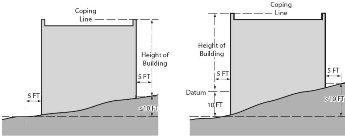
FIGURE 112-3B. BUILDING HEIGHT - PITCHED OR HIPPED ROOF
