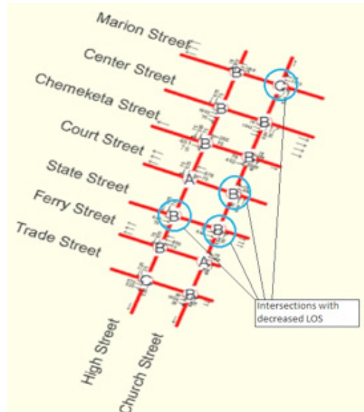
Figure 4: Synchro Level of Service results for System 2 analysis.
