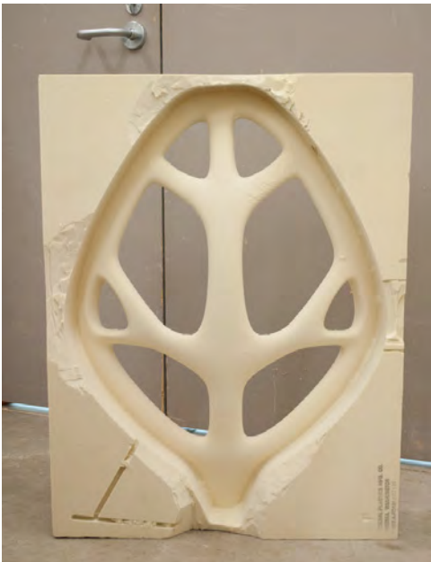
Figures 45 and 46: A model of the MELAS was milled out of foam on a CNC router
