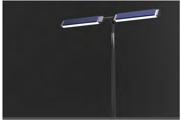
Figures 31 and 32: Renderings showing the solar panels on either side of the fixture
