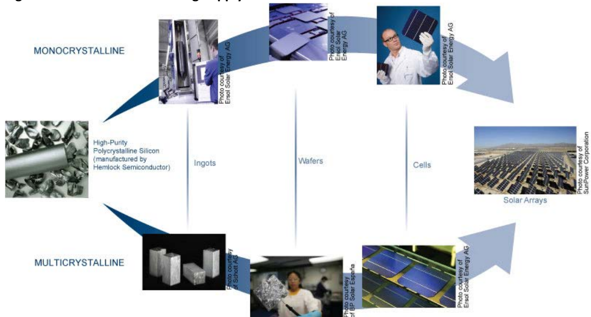
Figure G-3. Solar Manufacturing Supply Chain
