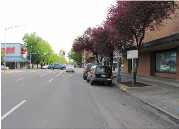
Figures 29 and 30: “Right Lane Must Turn Right” sign obstructed by tree on Liberty Street near intersection with Center Street; “Right Lane Must Turn Right” sign obstructed by construction vehicles on Liberty Street.
