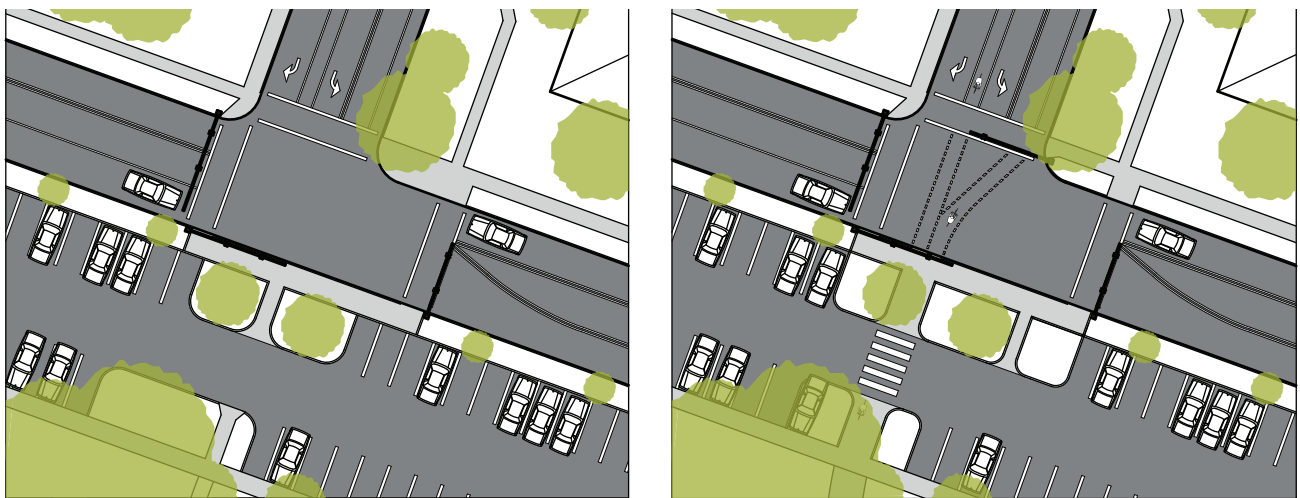
Figure 7: Before and after plans of the intersection of Winter and Mission Streets. Note widened shared use path entry to/ exit from Bush's Pasture Park, and street markings connecting cyclists to bike lanes already in place.
