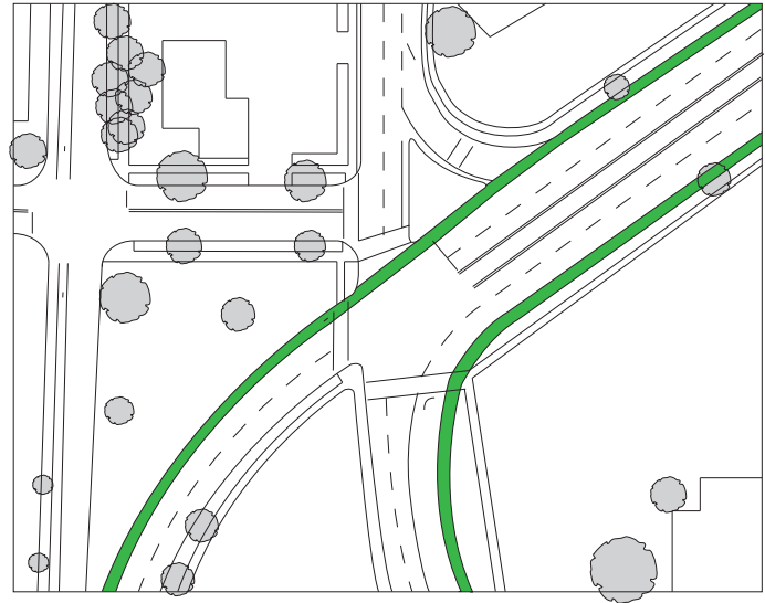
Figure 30: Proposed redesign with added bike lanes, and lanes extending across intersection, painted green to attract motorists attention. The median area between Salem Parkway, Tryon Street and Commercial could be used as a rest stop for cyclists, with a posted route map and bike rack.
