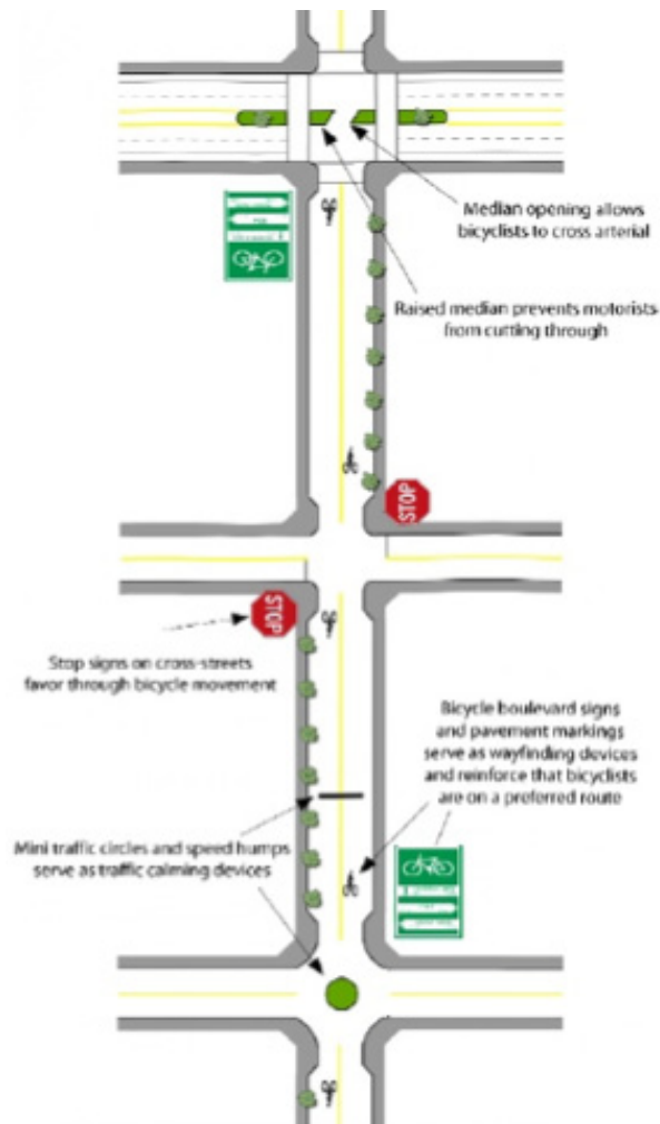
Figure 14: Design elements that may be used to develop a bicycle boulevard.
