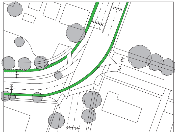
Figure 39: Proposed changes show connected bike lanes and bike lanes painted through the intersection.
