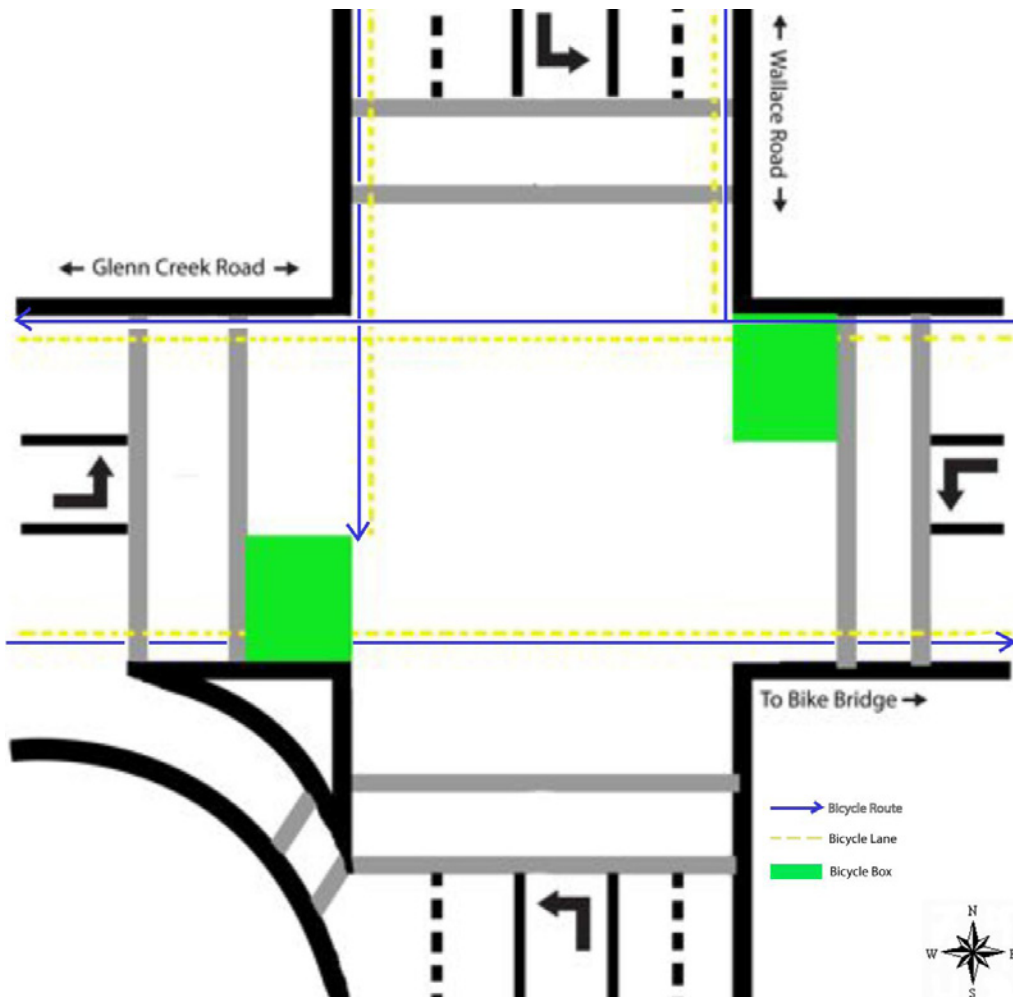
Figure 20: Two-stage bike queues place bike boxes in the east and west bound lanes of Glen Creek Road. Cyclists southbound on Wallace would cross to the Glen Creek bike box on the west side of the intersection and wait there for the signal on Glen Creek. It would take two phases of the traffic light for them to cross the intersection safely.
