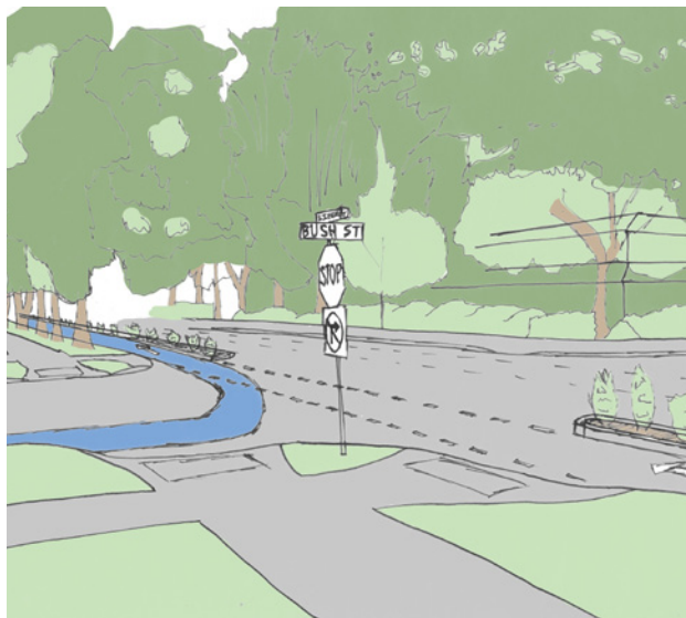
Figure 16: Image of intersection treatment at Bush Street and Liberty Street, with a painted, buffered bicycle lane merging onto the west side of Liberty Street.
