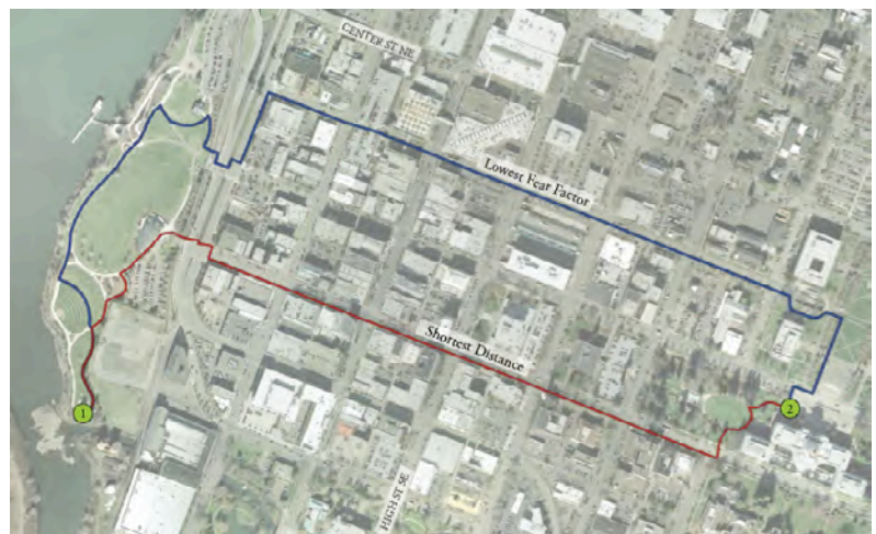
Figure 15: Bicycle Route Tool. The bicycle route tool calculates the shortest distance (red) or lowest fear factor (blue) route for bicycle travel in downtown Salem.
