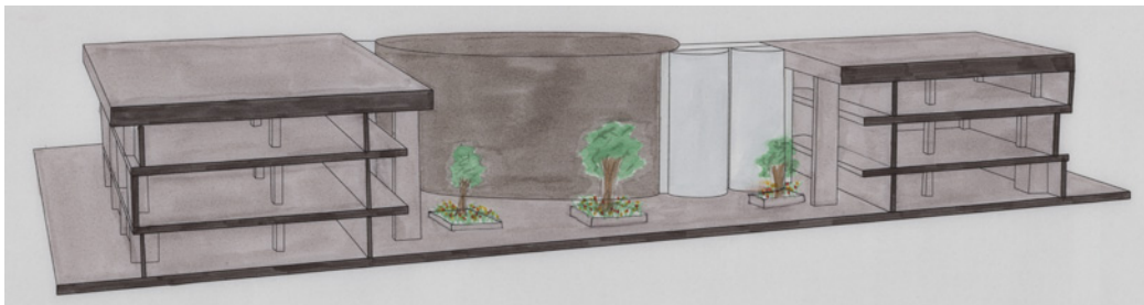
Figures 15 and 16: The atrium is not enclosed, but an additional structure provides large and small conference spaces as well as a space for the Council Chambers. This strategy creates a ceremonial space and scales the atrium while maintaining its original open character. (Madeline Brilliant)
