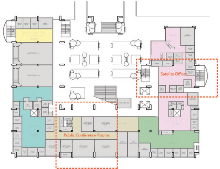
Figure 23: Satellite offices exist for each department that interacts with the public on the first floor. This way, quick questions and services can be accommodated easily, with internal vertical circulation connecting the satellite offices to the main departments. (Jamie Lundy)
