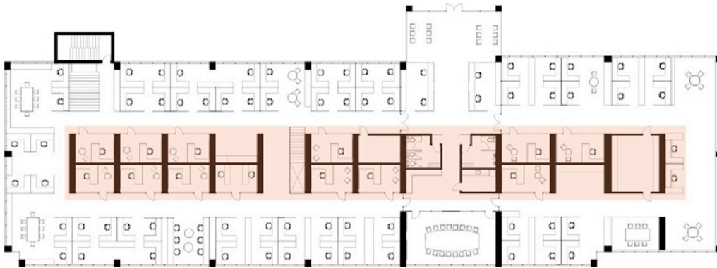
Figures 29 and 30: Closed offices, break rooms, and services create a core in the center of the department that serves the surrounding open office. This allows light to permeate through both sides of the department and reach the enclosed spaces in the center. (Marisa Baker)
