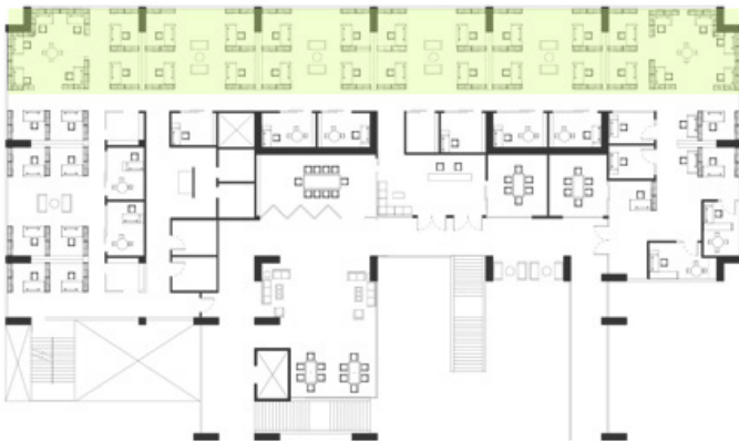
Figures 31 and 32: Meeting rooms are located on the most public side of the building (the atrium side), and open offices are located toward the exterior to allow for maximum daylight. Closed offices and services share a wall with the meeting room. This allows for a circulation spine and for light to permeate through the open office area. (Leah Fuller)
