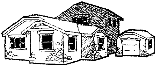
Two-story addition remains subordinate due to location, size and use of similar roof form.
