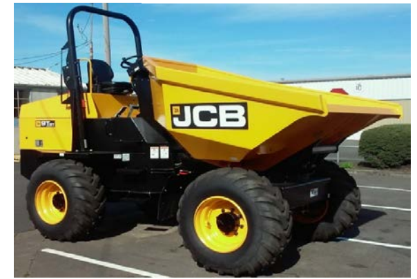
Below: This site dumper is used to replenish the slow sand filters at the Geren Island Water Treatment Plant.
