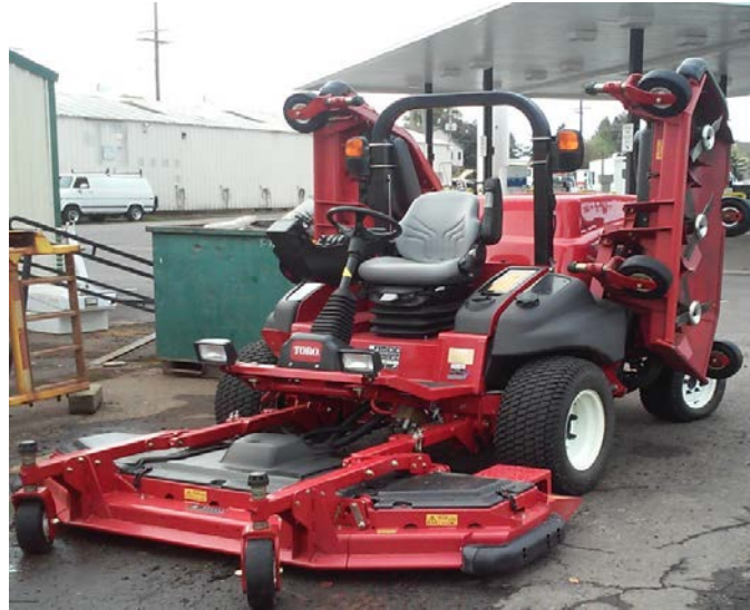
Left: The lawnmower, with its 16 foot mowing span, is used to maintain landscaping in some of the large regional parks in Salem.
