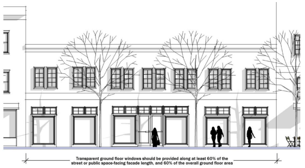
FIGURE 524-x. GROUND FLOOR WINDOWS
