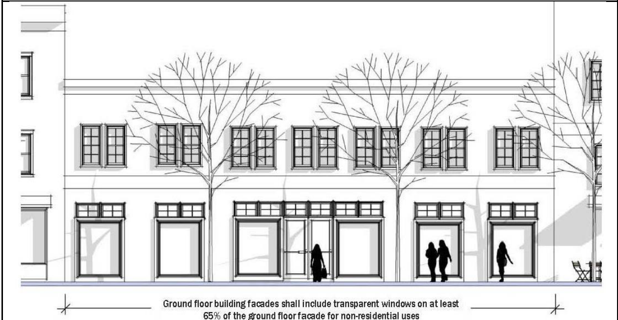
FIGURE 534-4 GROUND FLOOR WINDOWS
