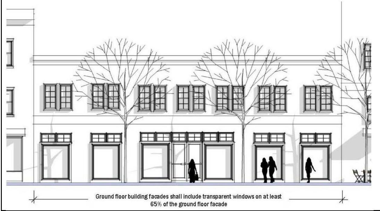
FIGURE 533-5 GROUND FLOOR WINDOWS
