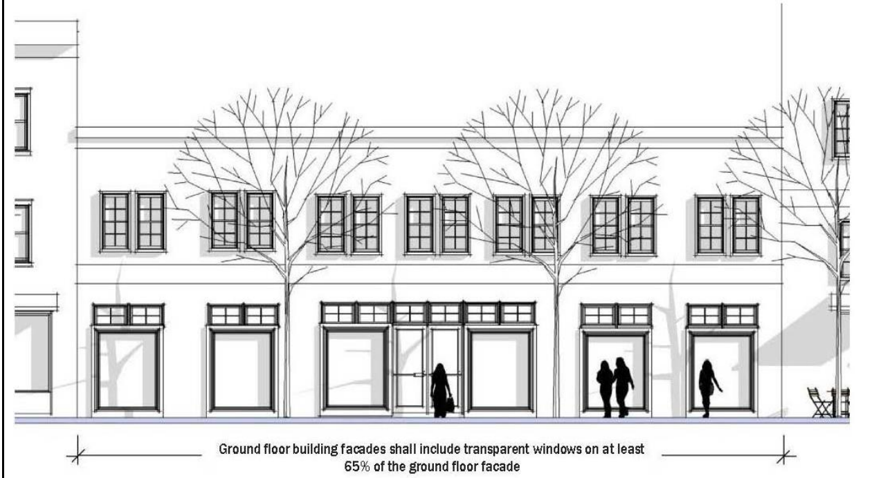
FIGURE 53X-5 GROUND FLOOR WINDOWS
