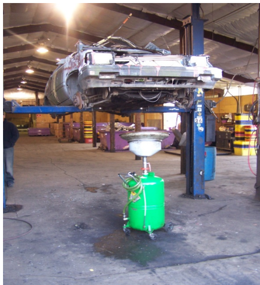
Fluid Gravity Drain System
